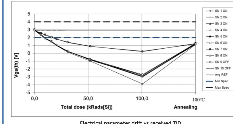
Electrical parameter drift vs received TID
