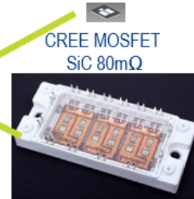
Same size as CREE 3-phase module L_{stray} = 30nH
