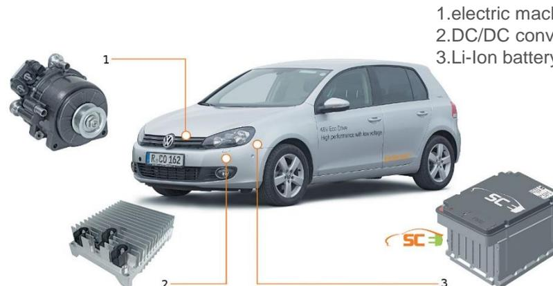
1. electric machine with integrated inverter
